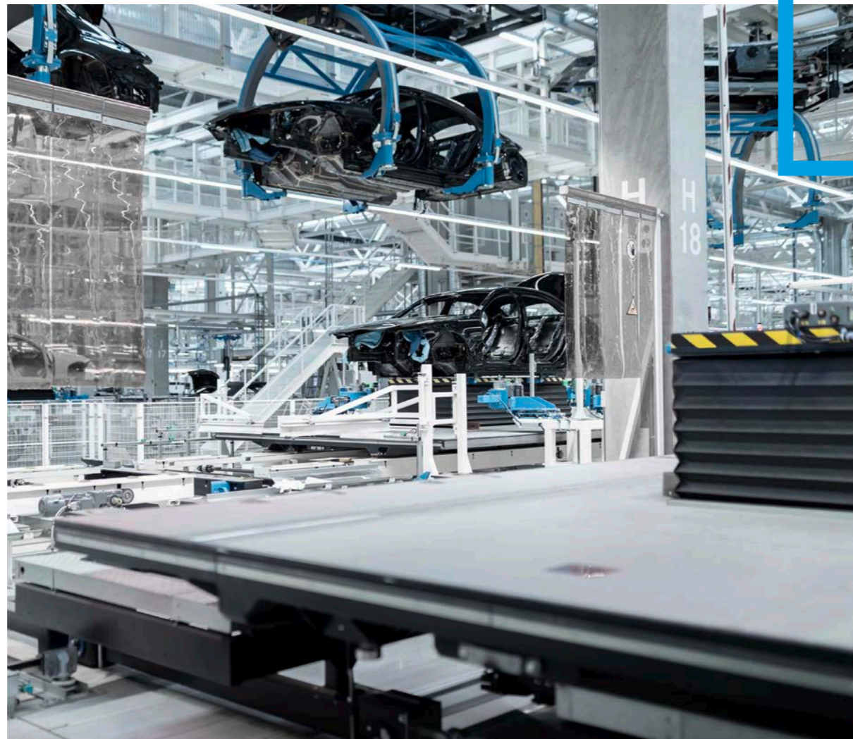
Skilnet platform with integrated lift table (bottom right) and heavy-duty EMS with integrated scissor lift (top middle) in a production environment
